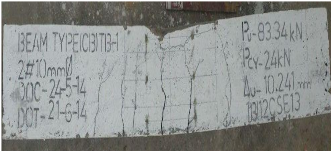
FIG 8: CRACK PATTERN OF TEST BEAMS
