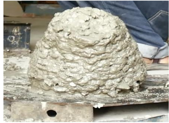
FIG 2: SLUMP TEST FOR FRESH CONCRETE
